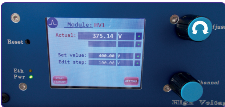
Figure 5: Operation mode – voltage adjustment.
